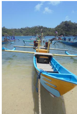
Figure 1. Traditional fishing boat with outrigger made of bamboo
